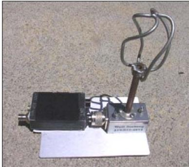
**Eggbeater Antenna.** No gain. Circular polarized in all directions: 360 degree. The box on the bottom has nothing in it, it is only a mount. The pictured one is for 1.2 GHz. This is a low gain CP antenna that gives good non-rolling pictures at short range. Of course it's a little fragile. It's a unique beast and not seen much because its hard to build. It works well. Great for car top, or boat, or plane bottom. **Price approx. \$ 400.00**
