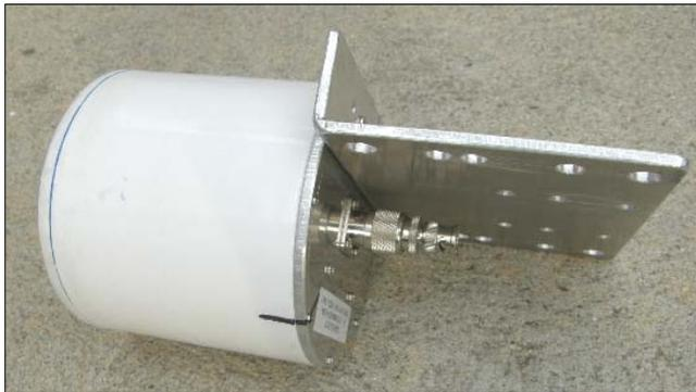
**900 MHz Cloverleaf** with shelf for Transmitter and holes for U-bolts to mount on pipes. Good for Coherent channels 7-0, this is a printed circuit antenna and it has slightly less bandwidth than the wired ones above.
