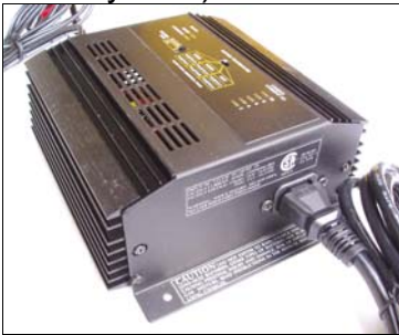
10A switching charger (little heat) 4A linear charger
