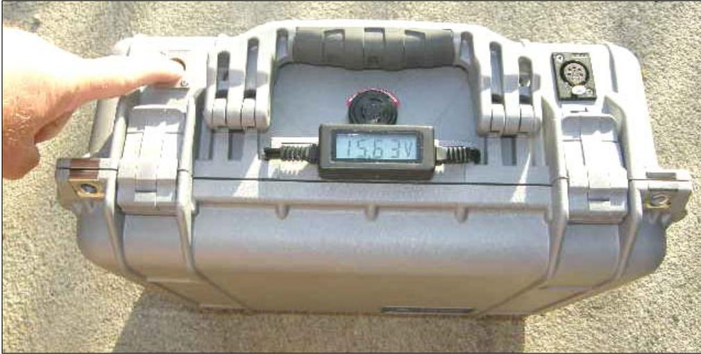
This economical battery **lasts 2 ¾ hr.** with all accessories powered up on the RED ONE™ camera. It recharges in 3½ hours.
