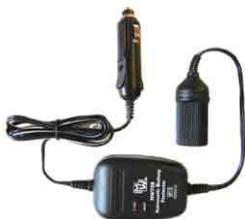
**Safety Cut off:** some older equipment, when running on batteries, does not disconnect from these batteries at 10.8 Volts. We have 10A and 60A cut offs that will save your battery from damage if you need them. Never overdischarge 12V Lead Acid type batteries lower than 10.8 volts, you will seriously reduce batteries lifetime. Take a battery down to 0 Volts and you may as well junk it. The same is true for
