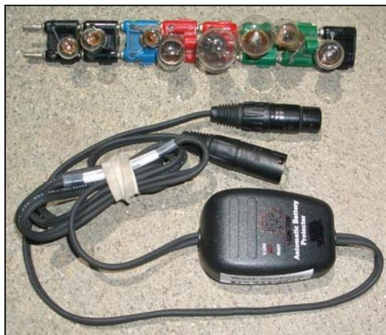
This is the voltage cut off good to 10 A and some load light bulbs. It is easy to assemble bulbs this way to come up with the load you want. The cut off protects the battery from over discharge. Just plug the thing in and go to bed.
