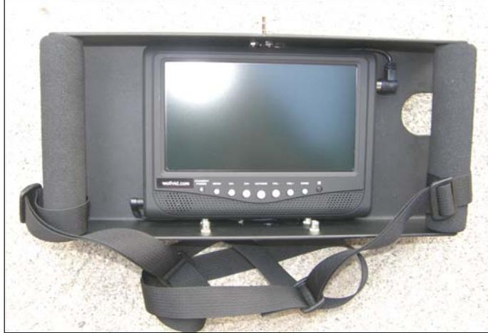
A bright monitor with digital + analog TV reception in combat-proof housing - receives signals from mini transmitters and broadcast TV stations, daylight viewable, NTSC: VHF, UHF, CATV, DIGITAL ATSC, 4x3, 16x9, not anamorphic, powers up on same channel as last powered down, Li-Ion NP-7L battery lasts 6 hours, attached in rear. Internal battery tested 1:45 hours.
